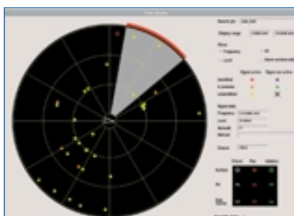
ESM**: displaying signals relative to one's own position in vehicles or on board ships
